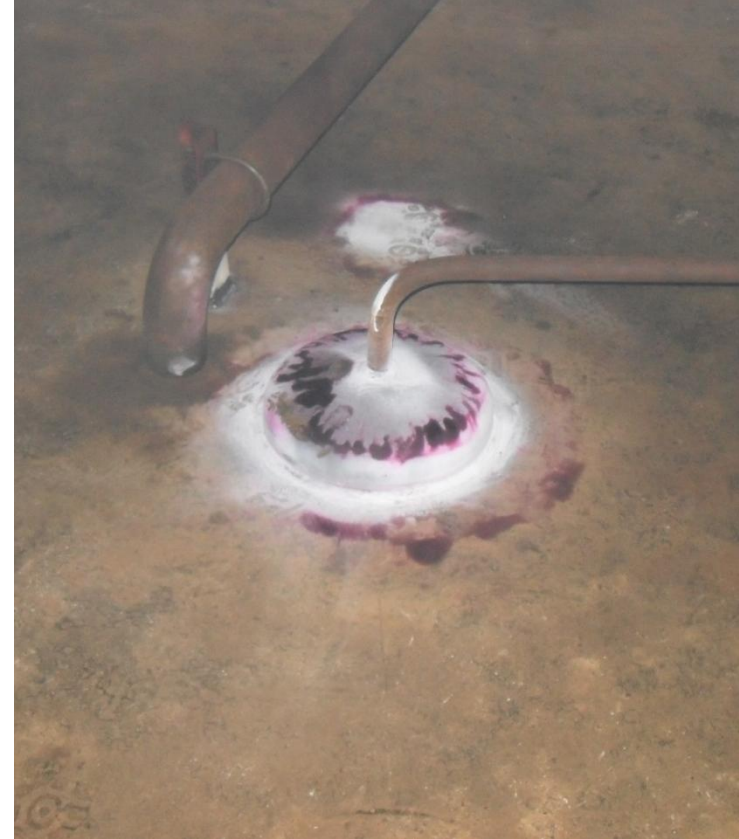
Measuring line connection at ground
